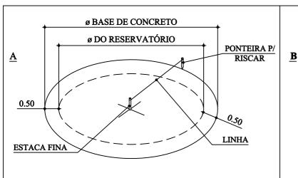
COMPACTADO E NIVELADO O SOLO, COM A AJUDA DE UMA LINHA AMARRADA A UMA ESTACA CENTRAL FIXA, TENDO NA OUTRA EXTREMIDADE UMA PONTEIRA, TRAÇA SE UMA CIRCUNFERÊNCIA IGUAL A DO RESERVATÓRIO MAIS UM METRO.
